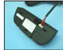
Figure 9 Connection of Power Cable
